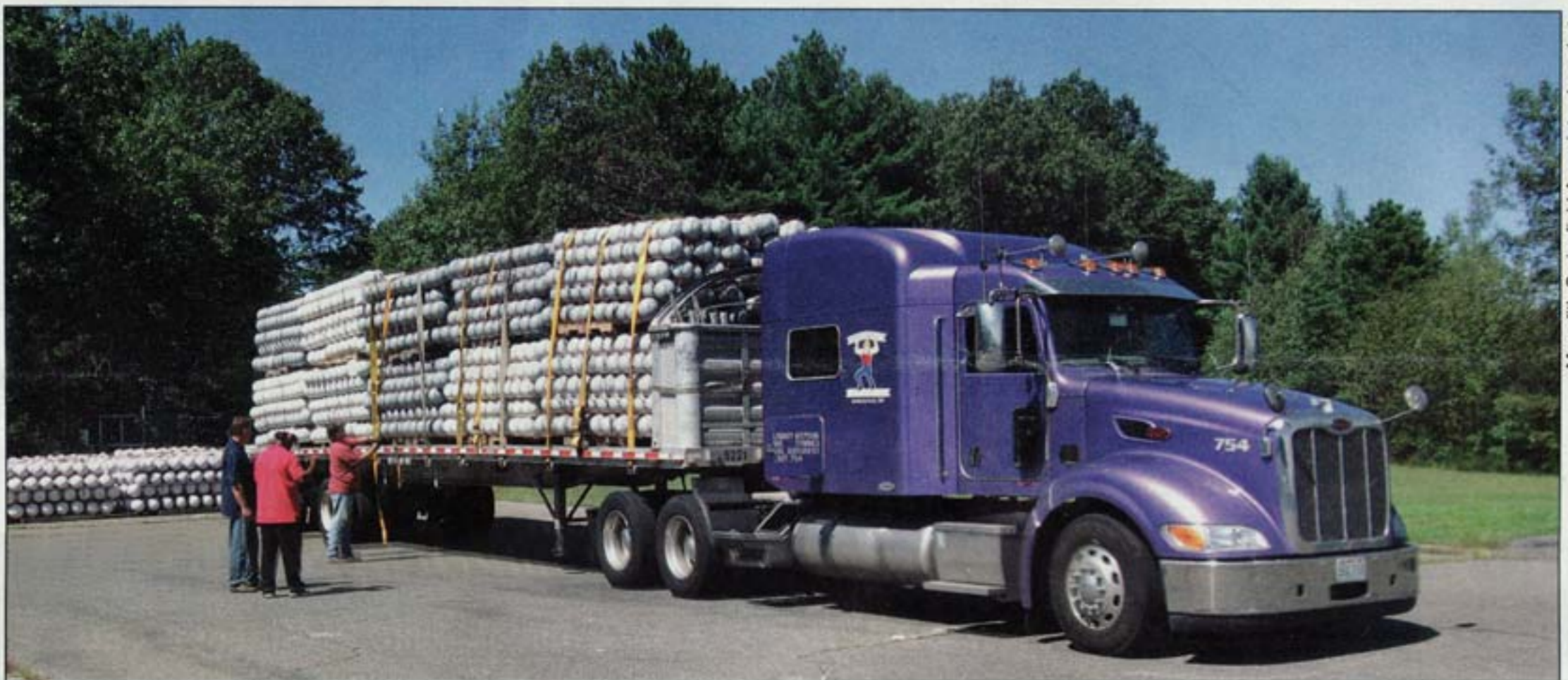
These plastic spheres will cut the amount of concrete needed for the Miami Art Museum, below, which is under construction.
